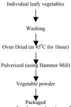
Fig 1: Flow diagram for the production of leafy vegetable powder
