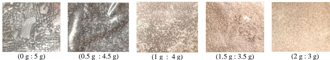
Figure 1. Bioplastic at different ratio of Jerbung shrimp waste powder and yam starch
