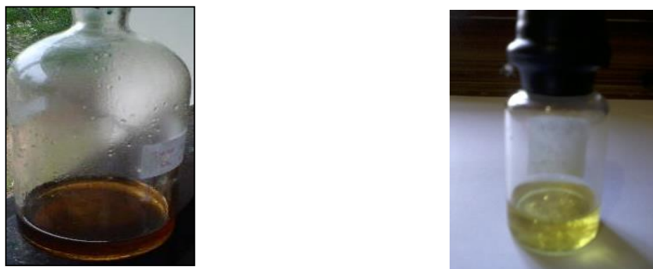
Figure 2. Oil liquid product (left) and distilled oil liquid product produced by catalytic cracking using H-USY
