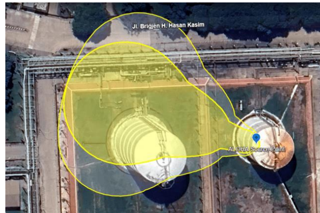
Figure 7. ALOHA Vapor Cloud Explosion Map Plotting for High Elevation Leak
