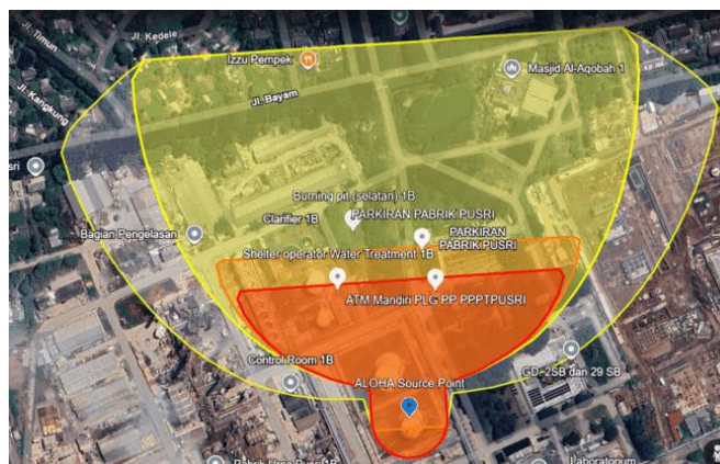
Figure 4. ALOHA Flammable Vapor Cloud Map Plotting for Low Elevation Leak
