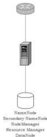
Gambar 2. Skema single node cluster
