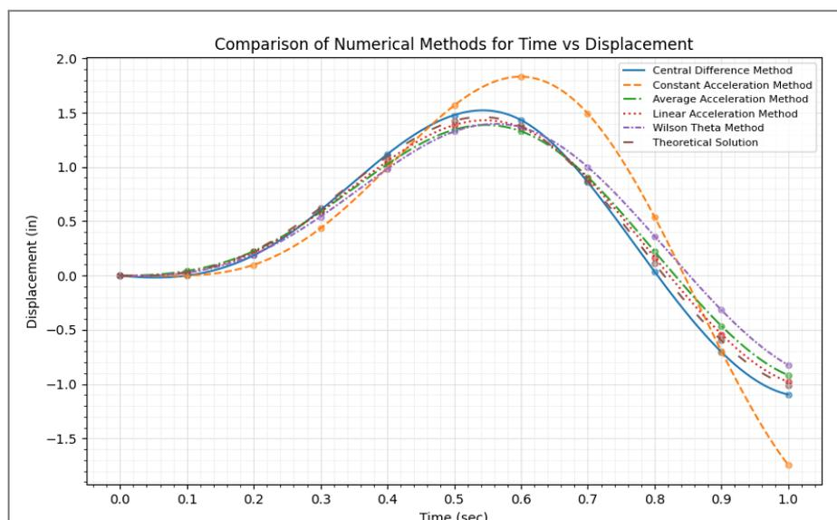
Figure 6. Comparison of theoretical displacement and displacement from each method
