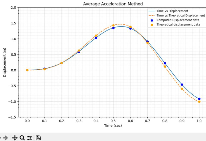
Figure 4. Comparison of theoretical displacement and displacement from Average Acceleration Method
