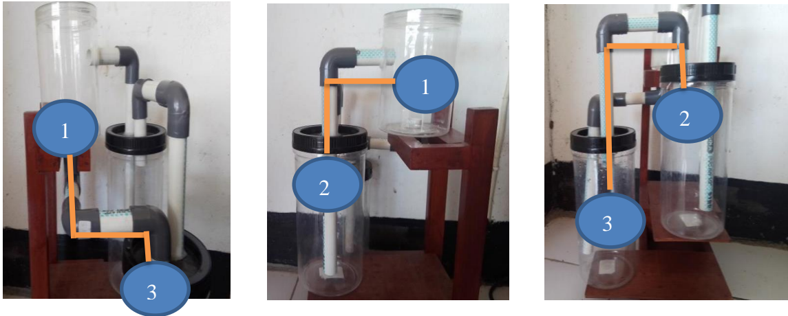
Figure 3. Installation of Pipes in Each Container
