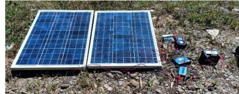
Gambar 2. Rangkain Seri 2 Panel Surya
