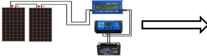
Gambar 1. Rangkain Seri 2 Panel Surya
