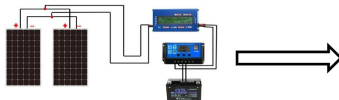
Gambar 3. Rangkain Paralel 2 Panel Surya
