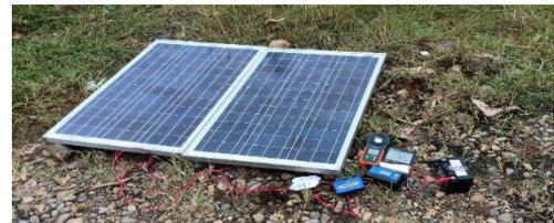
Gambar 4. Rangkain Paralel 2 Panel Surya
